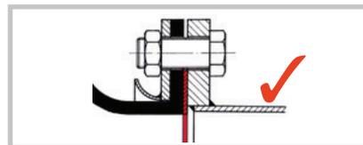
Additional flat seals (65<sup>±5</sup> Shore A) protect the rubber sealing face from sharp-edged pipe ends.
