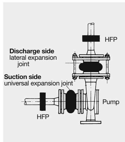
Recommendation for arranging expansion joints at pumps (normal case)
