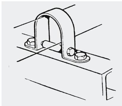
Pipe guide bearing with rollers
