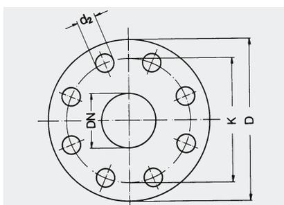
For pipes and fittings the screw holes must be placed in such a way as to be clear of the horizontal and vertical axes.
