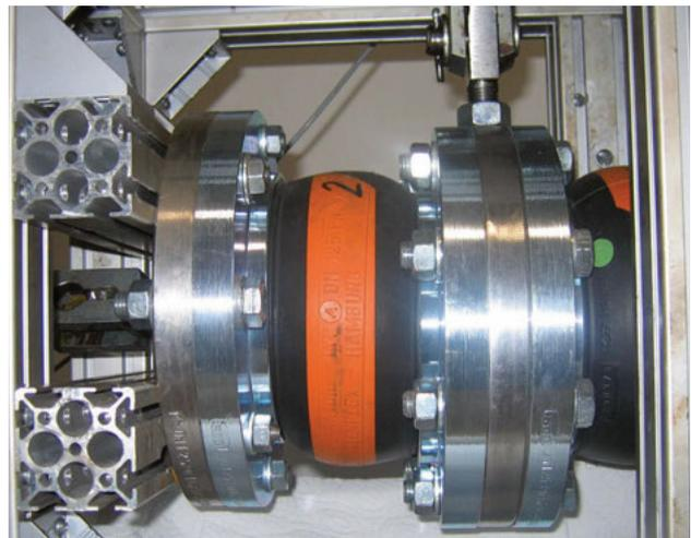
*On-going production monitoring of the expansion joints by load cycle testing machines*
