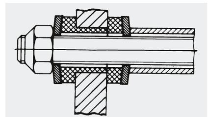
Tie rod restraints are carried in rubber sockets for sound absorption up to DN 150 as a standard feature
