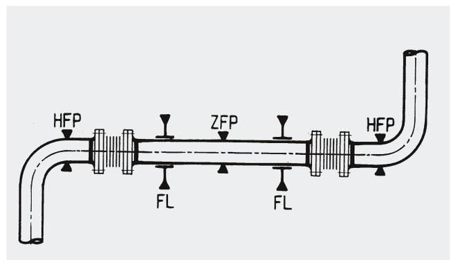
At pipe deflection points the main fixed points (HFP) and knee fixed points (KFP) absorb the full reaction force. The intermediate fixed points (ZFP) are practically relieved of pressure.
