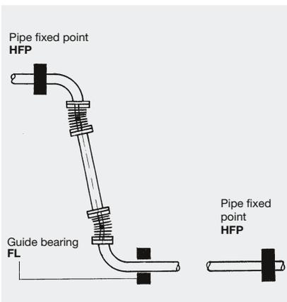
As a rule only one compensation system may be placed between two fixed points. When several compensation systems are fitted into the pipe system, fixed points must be provided between them.
